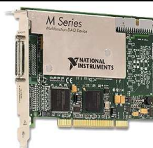
Carte d'acquisition National Instruments + Lab View
